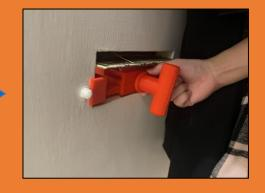
Then tighten the fixing ring on the handle to secure the entire holder
