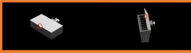
This parcel container NFC lock Located at the structure where the top lid protrudes. Users need use the type c cable to recharge their batteries, that kind of electric lock consumes little power and can be used for a very long time. You close the lid and it locks like a luggage locker. Only users and postman can easily open it. The postman can use their device touch to NFC LOCK to open and drop off parcels. The user can use the app on the phone or use NFC to open the parcel manager.
