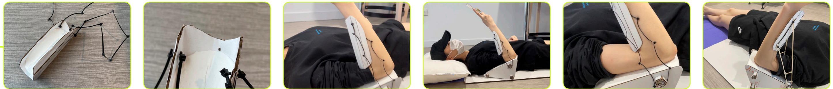
There is a layer of cushion inside part of the arm, which can better fit the human body. But the first 'pull type' of force is not reasonable. The piece holding the arm will fall down and get stuck on the arm.
