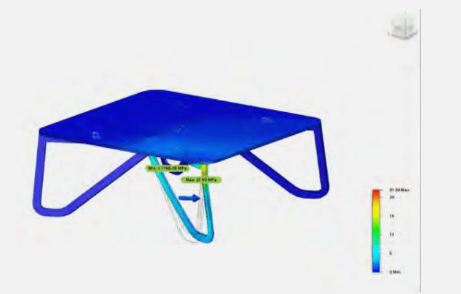
Maximum Stress in 9mm Plywood with 25mm leg width and 10kg point load
