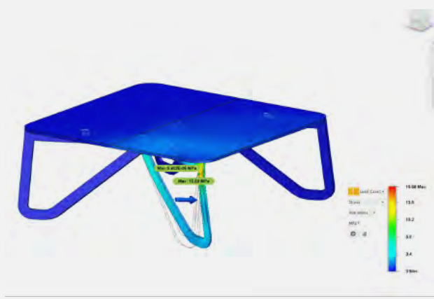
Maximum Stress in 9mm Plywood with 30mm leg width and 10kg point load
