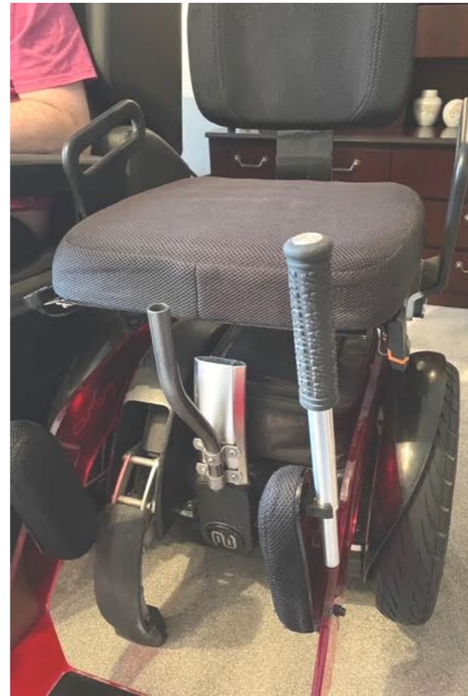
Handle stored in side holster, allowing for unobstructed transfer
