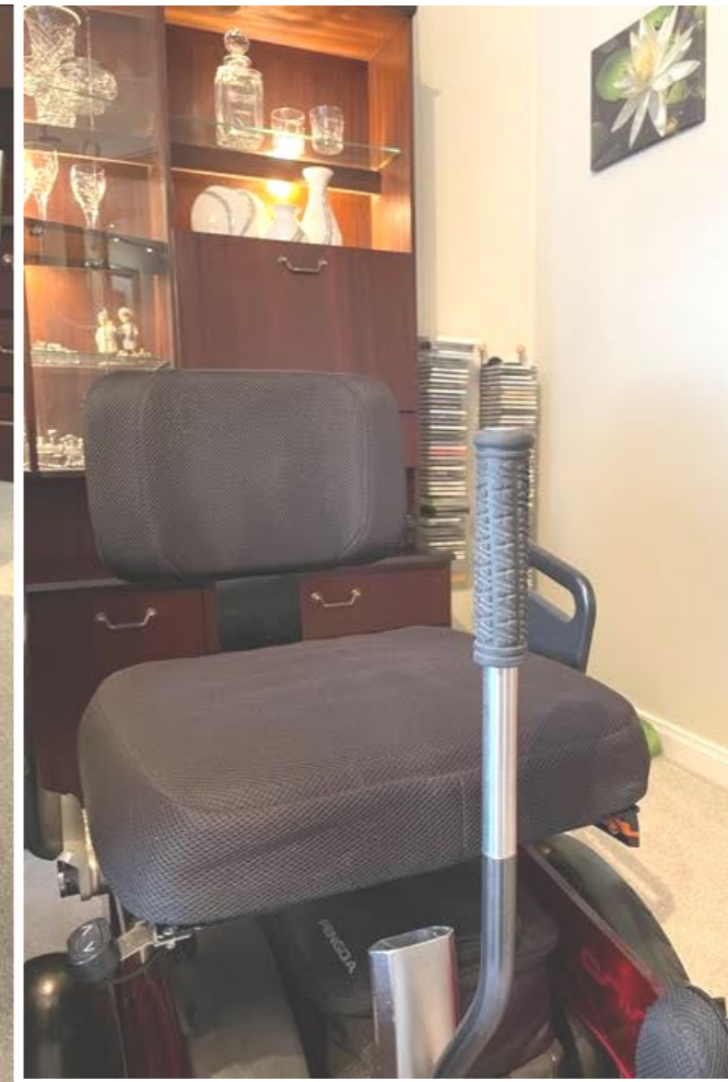
Handle inserted into stem, ready to use for steering
