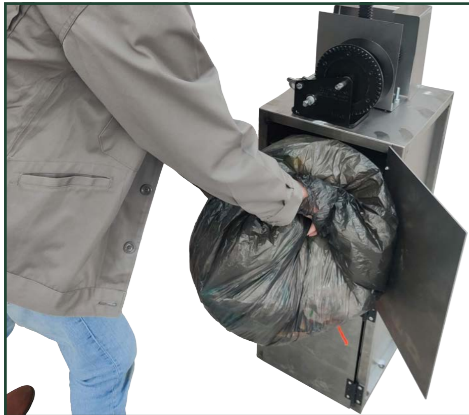
1. Insert bagged soft plastics into baler
