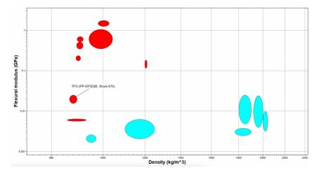
TPO Shore A75 was chosen as the elastomer material after considering each material's injection moulding capabilities, weatherability, and Shore A hardnesses. A material which had similar properties to Sugru was desired because of the large amount of positive feedback the physical prototype generated. Online research also revealed that ABS and TPO is typically used in two step injection moulding products.
