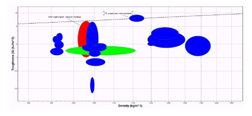
ABS is a light, high impact material which is widely used in an array of product applications. It is low cost, and perfect for mass manufacturing through injection moulding.
