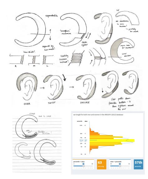
The challenge with the expandable leg was creating a mechanism which deformed sufficiently over a long number of cycles, yet was still able to apply a light pressure to the ear lobe. The final prototyped mechanism was made of wire and Sugru and was deemed a comfortable, yet secure fit.
