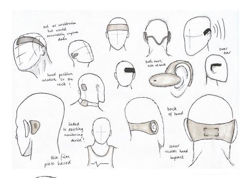
The main challenged faced early in the concept generation process was the balance between obtrusive and completely 'invisible' designs. The further to the left of this scale meant the less reliable the impact data would potentially be and less personalised to each player. Too far right on the scale however would have too much effect on the user, even though the data would be robust.
