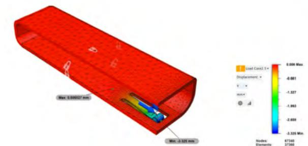
The width and length of the snap fit were varied, and the optimum length was chosen as 25mm, and the width as 5mm.
