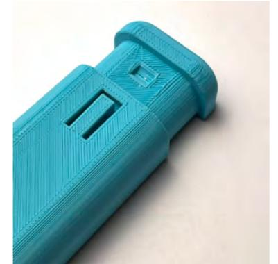
To develop the optimum snap fit size, several Fusion360 force studies were conducted, which tracked the displacement, stress and relevant safety factor for a variety of loading forces.
