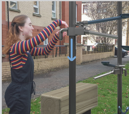
Vertical translation down the shaft, locks in place through push-release mechanism in primary handle
