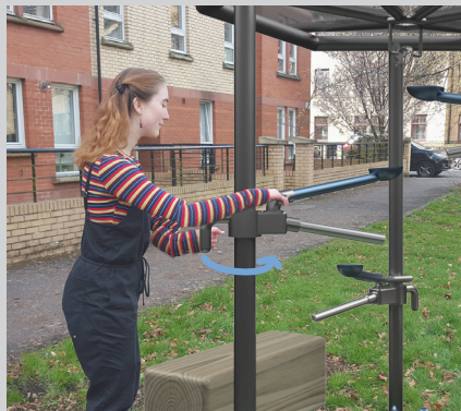
Rotation about the shaft through the main handle, restricted to 60° of motion
