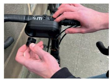
**3.** The front light is attached to the handle bars and it recognises the polarity in the front mount, automatically turning the light white.
