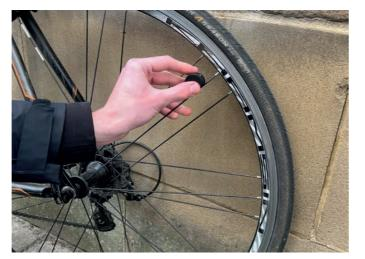
**6.** Upon removal from case the spoke lights automatically turn orange indicating side visibility mode has been activated.
