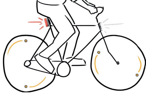
Assuming POV is achieved at  $\tau = \frac{1}{10}$  or f = 10 Hz@ wheel = 622mm C = TED = TE - 622×103 = 1.95m 1609.34 m in a mile 1.95 m/5 . 3600 slbs = 7020 m/hr For the wheel to rotate with a frequency = 1 Hz it must travel  $7020 \cdot \frac{1}{1609.34} = 4.3 \text{ mph}$ 18 there was 2 lights per wheel the cyclift would need to travel ~21 mph!
