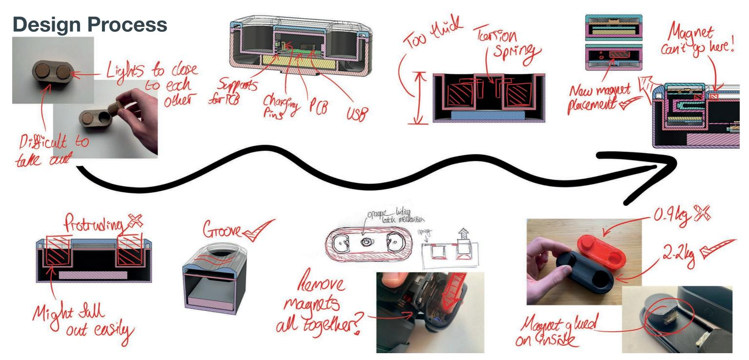
After the design of the spoke light had been finalised, a cardboard prototype was created to get a sense of the overall scale of the product. This highlighted an issue with taking the spoke lights out of the case. I hadn't considered that they would be sitting flush with the main light so there was no where to grab onto.
