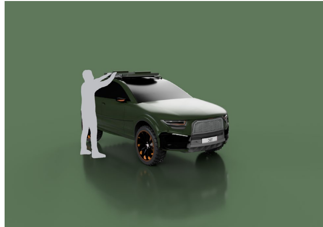
The base is lifted onto the vehicle roof and attached in four locations.
