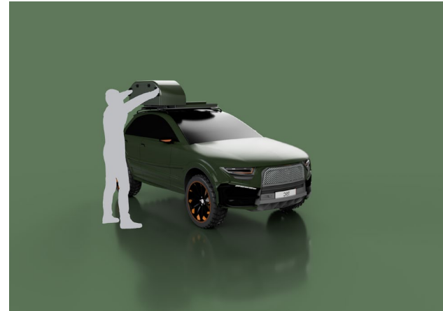
Container one is lifted, placed and then slid onto the dovetail runners until it reaches the desired position.
