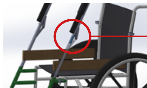
Spring loaded latch to Lock hinge and align pipes
