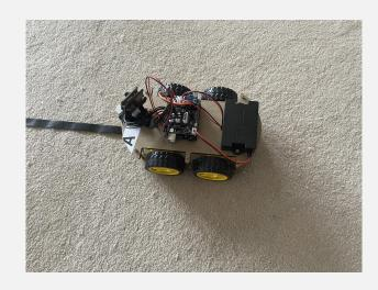
When the distance between the front object is less than 10, it will automatically avoid
