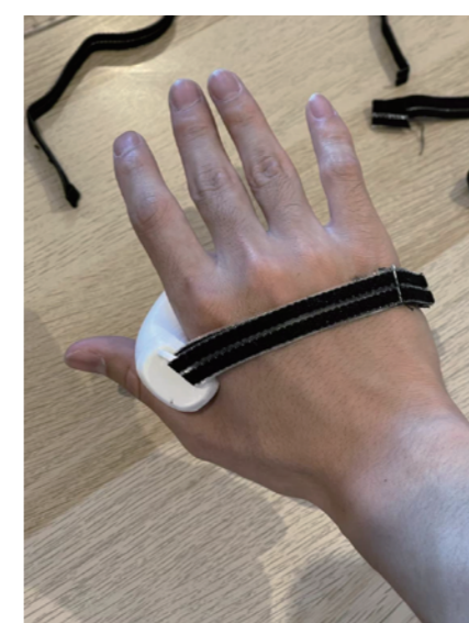
After testing, a model of the product is made using 3D printing and demonstrates how the user uses the product in their hands.
