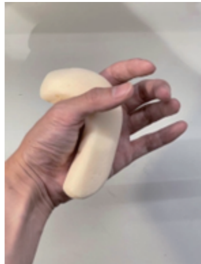
Use foam prototypes to test different sizes and comfort, select the thickness and radian that most easily fit the hand, and test the use angle and effect of the adjustable tape.
