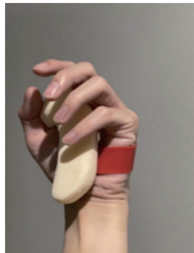
Use foam prototypes to test different sizes and comfort, select the thickness and radian that most easily fit the hand, and test the use angle and effect of the adjustable tape.
