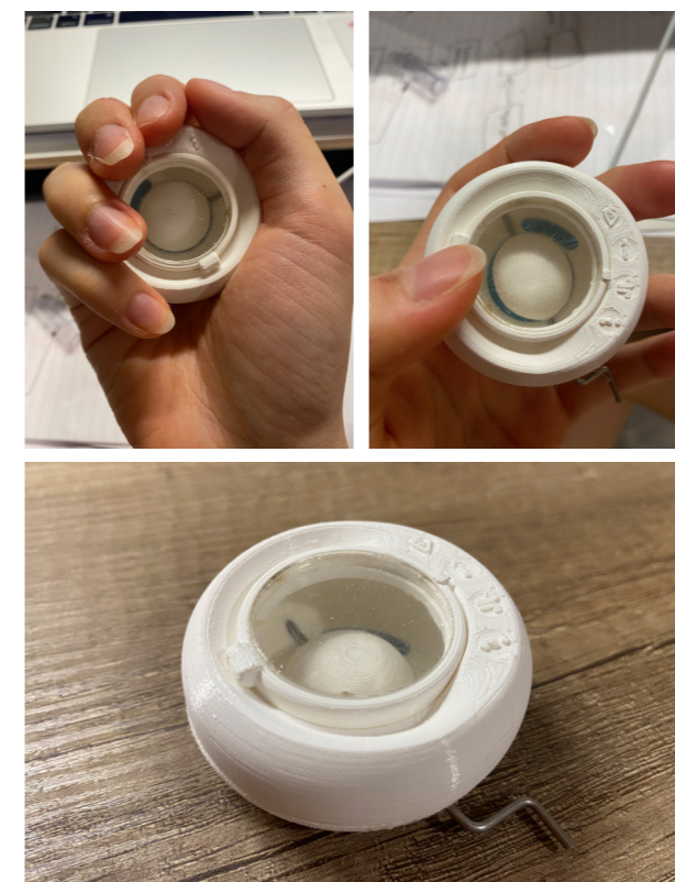
Silicone layer attached
