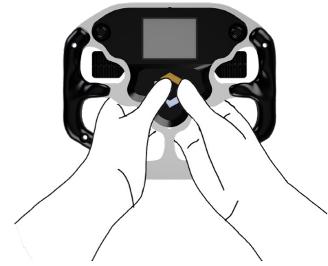
Two-handed access through the inner hand spacing in the base plate
