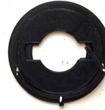
Failed due to lack of guides
