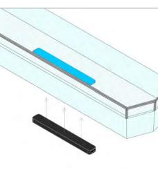
The dock is then magnetised to the mount on the underside of the tray.
