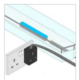
The power cable is connected to the dock and run to a plug socket.
