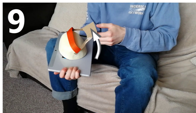
Lever lifted from underneath, detaching product
