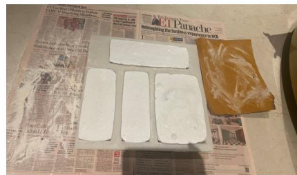
7. Sanded the mold- this will be used to give thickness to compartments
