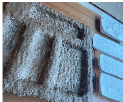
8. Poured the slurry (cardboard + water) and gave thickness by pressing the mold
