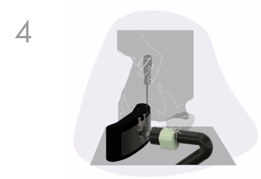
4 The workshop engineer attach on an external head pad onto the mount, using the ball joint. This is clamped together.
