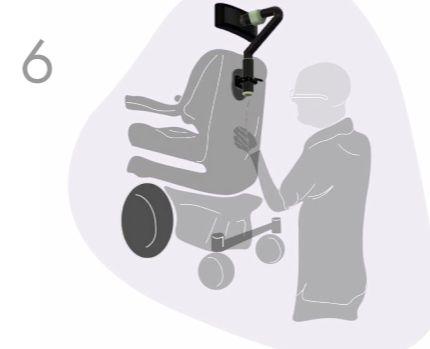
6 The headrest is clamped into the mounting bracket and plugged into the power module located at the bottom of the chair
