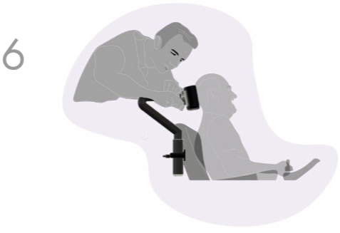
6 The wheelchair batteries go flat on the wheelchair but Bill wants the headrest rolled back. His son Ben can do this by releasing the headrest pad from the ball joint and manually moving it
