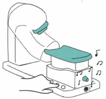
To replicate the sound of the machine, a small speaker is position on the Linac base. The patient simply pushes the button for 10s of sound play.
