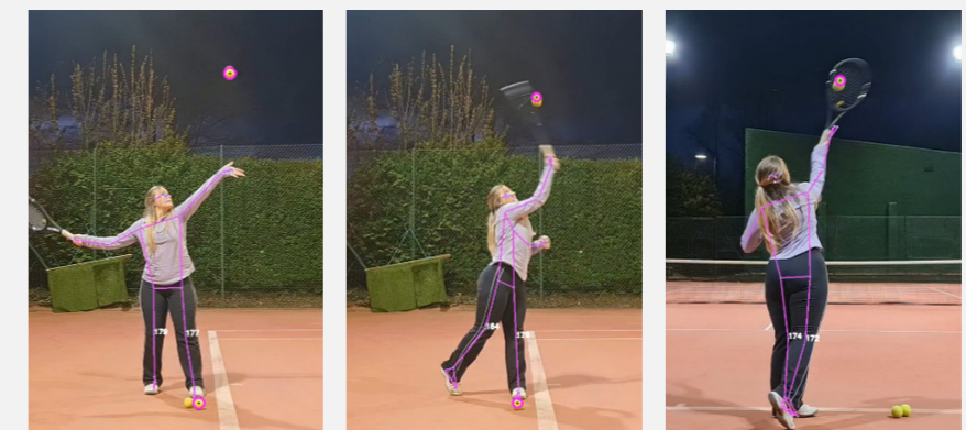
Human pose estimation using SONY IMX 477
