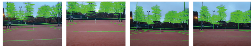
Experimental output of the line detection software. Detection accuracy increased as the height off the ground increased.
